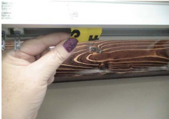
6. Make sure the pinion rod is fully seated in the control mechanism. If not, slide the pinion rod into the control mechanism, turning the rod slightly if needed.
