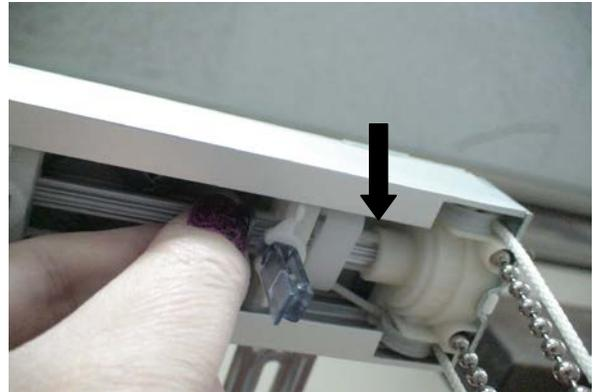
7. There may not be enough lubricant on the pinion rod. Spray the pinion rod with a water-based silicon spray. For approved silicon sprays, see step 10.
