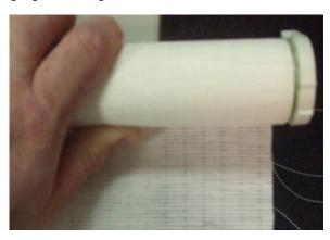
**6.** While keeping the shade completely rolled, reinstall shade starting with control end. Ensure the latch on the non-control end is open, then place into notch, close lever.
