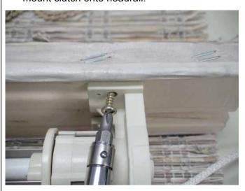
**12.** Make sure cord clips are evenly spaced from shaft bracket. It is important the lift cord starts on the back line located on the shaft.
