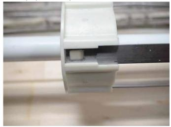
**10.** Tighten screws to attach the retainer disc back onto the shaft.
