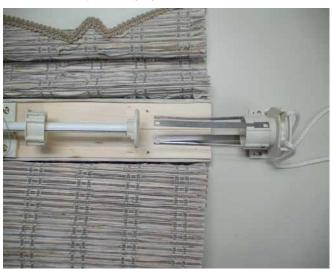
**4.** Remove disc from end of shaft by removing the screws, then remove retainer.
