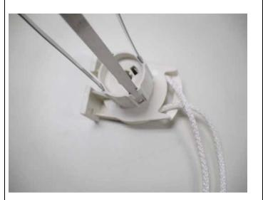
7. Slide NEW retainer into shaft.
