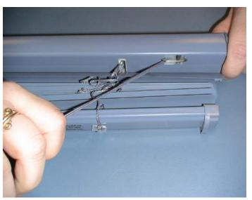
15. If the blind has two lift cords, follow steps 15-20 to attach the clear cord stop beads. If the blind has three or more lift cords, follow steps 21-22 to attach a safety joiner ball. Create a loop in one cord just below the headrail insert loop into a cord stop bead and position the bead approximately 2" to 3" below the headrail.
