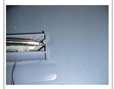
**4.** Push the tilt rod away from the cord lock just far enough to allow room to work. Be careful not to push the tilt rod past the tape drum as this could make the blind inoperable.
