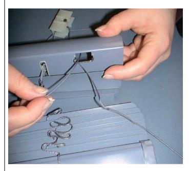
**10.** Turn cord lock right side up. Be sure to hold the rivet in place. To install the replacement cord lock, slide the front of the cord lock under the lip in the front of the headrail until it is positioned over the hole.
