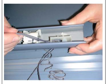
**6.** Place needlenose pliers inside the cord lock and push towards the back of the headrail. The cord lock should disengage.
