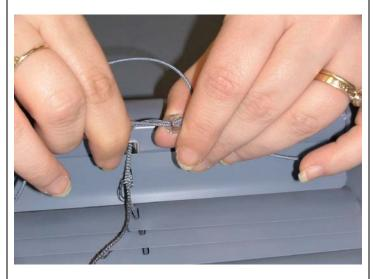
**20.** Hold cord stop bead in place and pull firmly on pull cord to re-tighten knot. Repeat each step for each stop bead.
