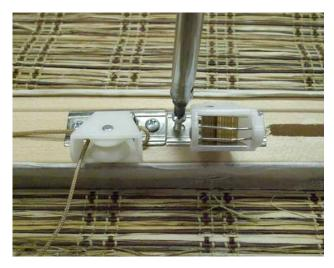
**10.** Thread the cords between the rollers inside the cordlock and on either side of metal cord separator.
