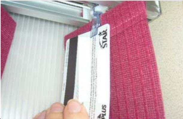
2. Remove louver by pulling down on both the louver and the plastic card at the same time. Lay louver on a clean flat surface. Repeat for all louvers.
