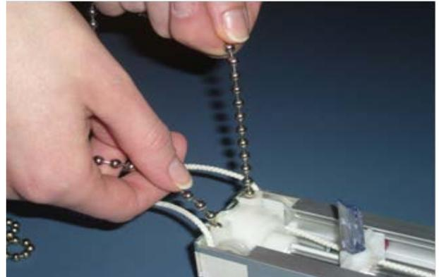
7. Once you have confirmed that the headrail is operating properly, reinstall the headrail into the mounting clips and rehang the louvers with the stems in the open position. All louvers should be facing the same direction.
